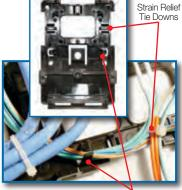
Single/Double Gang Electrical Box Mounting Holes
